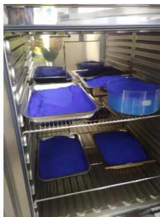
Figure 1: MOFs (HKUST-1) beads of 80 µm in diameter prepared by spray-drying process
